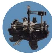
**Available with:** up to 6 micro-manipulated probe arms • temperatures from 1.6 K to 675 K • cryogen-free cooling • vertical or horizontal field magnets up to 3 T • up to 4-inch wafer probing • high vacuum to  $10^{-7}$  torr • DC to 67 GHz measurement – coming soon: a THz arm for 75 GHz & up
